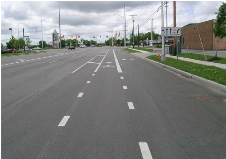
Bike lane in Hilliard, Ohio showing the markings at an intersection with a dedicated right turn lane.
